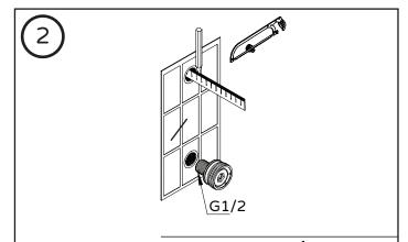
Measure the depth of the inner thread of hot & cold water pipes. This is to assure that there is no gap between the wall and brass connector. The fitting should be recessed into the wall 3/8th's to 1/2 inch from the finished wall surface
