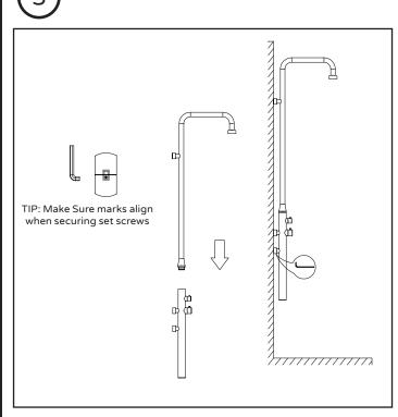
Insert upper shower to the lower shower. Make sure the marks align on the pipes, then lock and screw the pipes.
