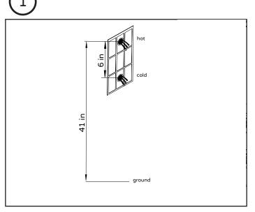
Install the Hot & cold water pipes at 41 inches\* from floor surface to the top water(hot) outlet. Flush the pipes before installation. Make sure the distance between the two pipes is 6 inches, and allow some room for adjustment.
