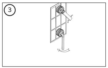
Apply teflon (plumbers) tape. Tighten the two brass connectors to the hot & cold water pipes.
